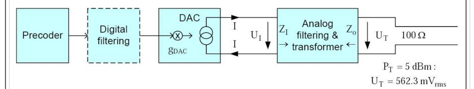
$Baseline \ approach: \quad I = 15.9 \ mA_{rms}, \ \ U_I = 891.1 \ mV_{rms,diff} \quad \stackrel{\Delta}{=} \quad V_{CT} \pm 445 \ mV_{rms}$
